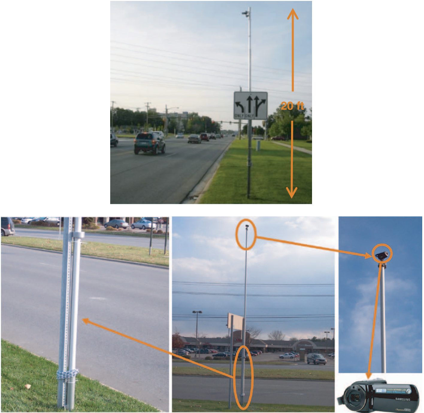
Figure 3. Field setup for video recording of driver behavior data.
